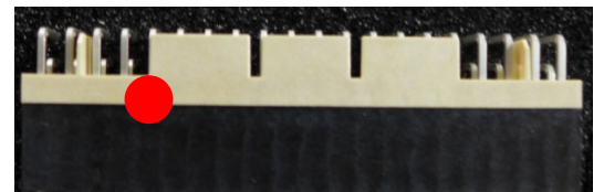
Figure 6: "Approximately Hottest Spot", 10 Contacts in Linear Series
