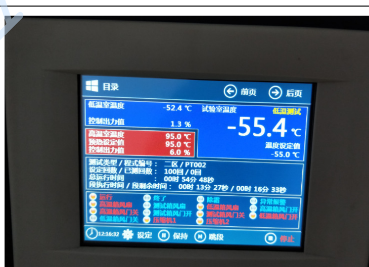
Figure 2: The setting test condition parameters
